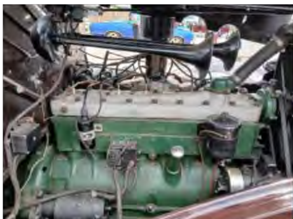
280 c.i. inline (4.6 L) flathead 8 cylinder, aluminum head, shaft driven supercharger. Certainly this block contributed substantially to the 3,840 lbs weight of the car.
