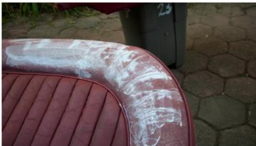
crack filler sanded
