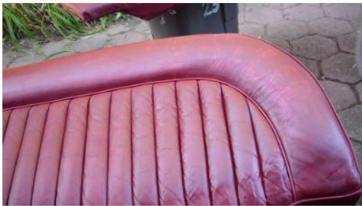
1 st coat of leatherique dye added
