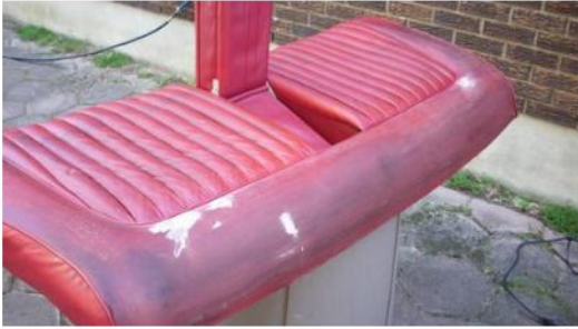
old dye removed and crack filler
