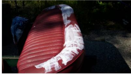
old dye removed and crack filler
