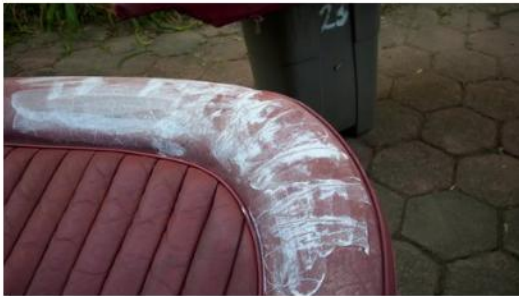
crack filler sanded
