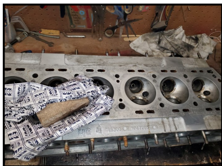
Decking the Head
