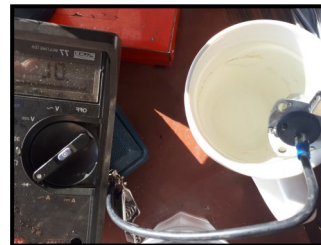
Testing AED Switch
