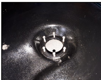
Tank now ready for new fuel sender
