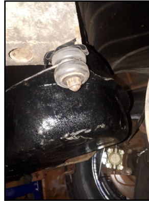
Rebuilt fuel tank & mounts
