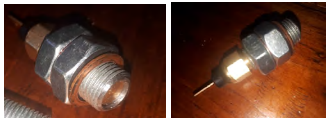
Showing oil temp sensor adaptor. \frac{1}{2} " UNF & female \frac{1}{8} " NPT.
