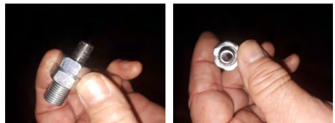
Showing the oil pressure sensor adaptor. Note my lucky off center drilling. \frac{1}{2} " UNF & male \frac{1}{8} " NPT.
