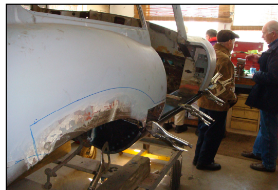
Clamped in place for welding
