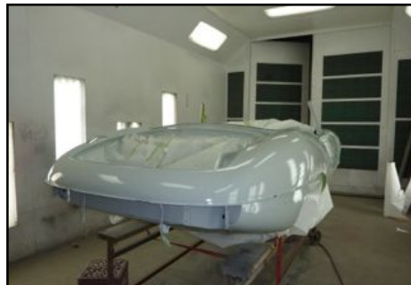
Primered and ready for paint
