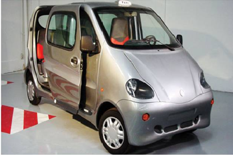
This six-seater taxi, which should be available in India next year, is powered entirely by a tank filled with compressed air.
