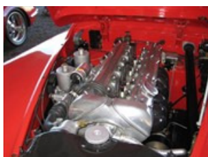
Early XK120 With Studless Cam Covers and Sandcase SU Carbs
