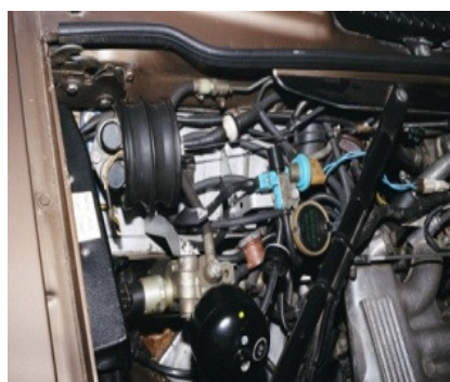
Figure 1: The relocated cruise control bellows.
