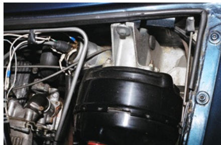
Figure 3: The new HT coil location.
