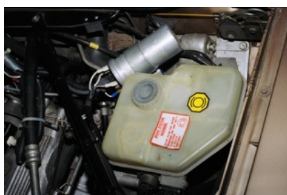
Figure 2: The relocated HT coil.
