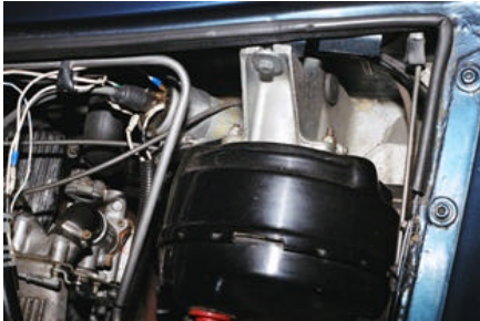
Figure 3: the new HT coil location
