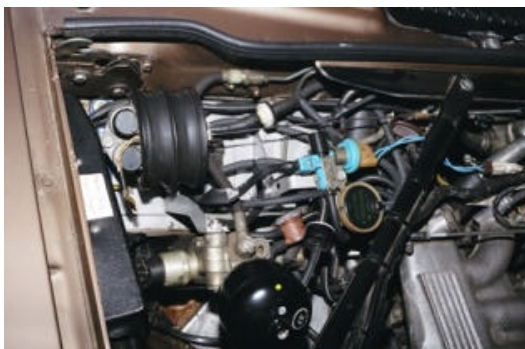
Figure 1: the relocated cruise control bellows
