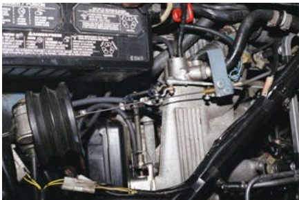
Figure 4: the new location of the cruise control bellows
