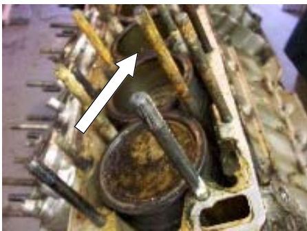
Calcium deposits are apparent on the second stud.
