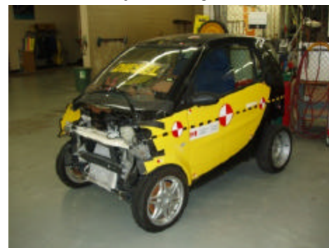
A Smart Car after crash testing; not much left of that front end, but the rest was in fairly good shape.
