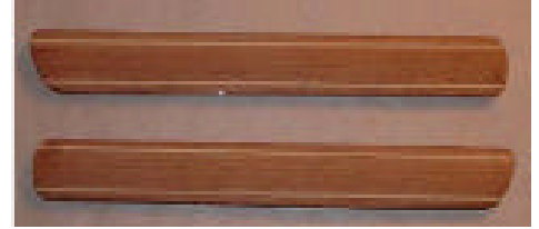
Side panels sanded - ready for veneer joining pieces – meant my wood grain might not flow as nicely as desired.
