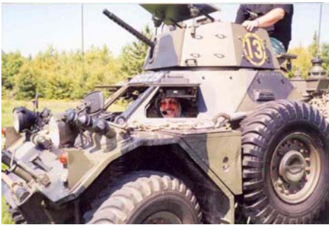
Pete driving a Daimler Ferret armoured car; even with a Rolls Royce 6-cyl 129 hp engine, it has a maximum road speed of 93 kph. Definitely not the Mk2!
